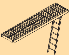
Aluminium platform with ladder (aluminium/wooden)
