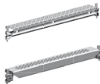
U-gap decks/U-ledgers with gap cover, 0.11 m wide are available in a variety of lengths for gap-free work surfaces between U-main scaffolding decks and U-console bracket decks (see pages 42 / 43).
